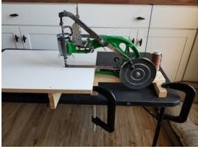
It comes with a worthless tripod stand so I made my own from wood. See the pictures. It is a cylinder arm machine with a walking foot with a rare feature. The walking foot can be rotated in any direction;
