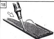
Round the edges of the leather on both sides with a bevel-eze edge beveler.
