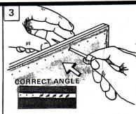
Stab first hole with awl as shown above. Be sure to stab proper angle with the awl blade.
