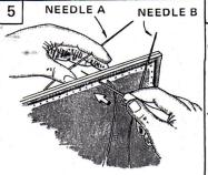
Punch second hole with awl. Hold needles as shown above.
