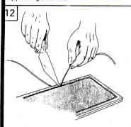
Cut threads off in stitching channel on both sides with a sharp knife.
