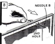
When putting needle "B" through always put it on the same side of thread "A". This will insure uniform appearing stitches.
